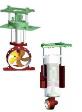
NTA twin screw azimuth thruster
